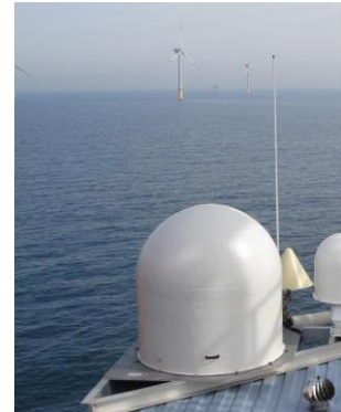
Figure 2c. BirdScan MT1 has been used by Schulz et al. (2014) at Alpha Ventus. It was situated at the FINO1 research platform.
